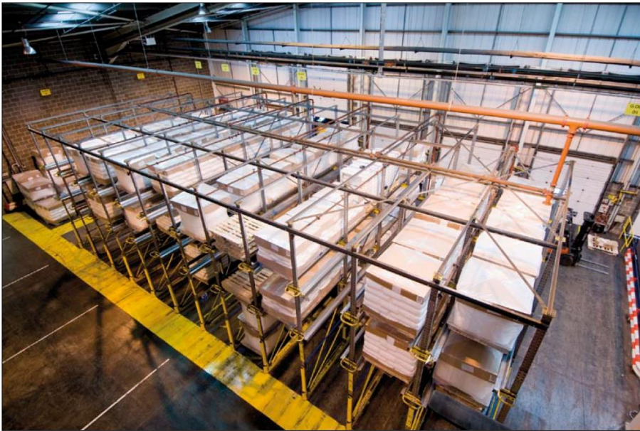
Storage of packaged dangerous goods in racking
